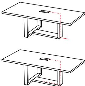
The distribution of the electricity is entirely configurable; the exit for the cables can be placed on the left or the right side and be made to be placed on the interior or the exterior of the table.
